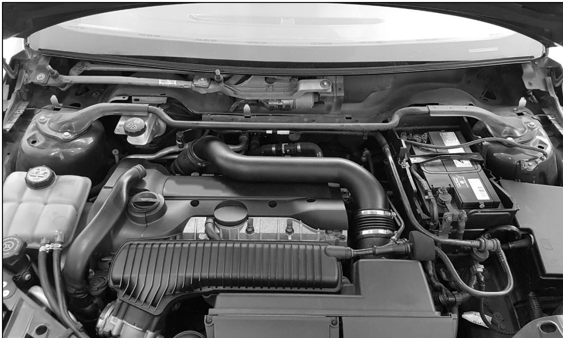
Pictured above is the engine bay with the lower cowl panel removed and factory strut brace in place.
